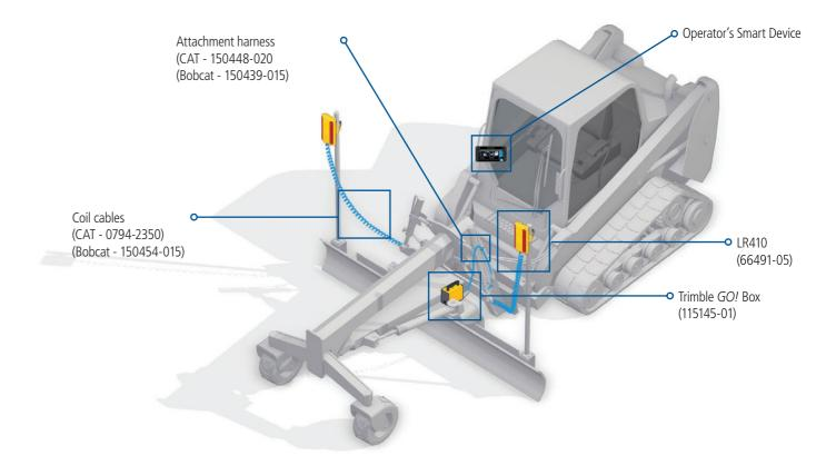
Trimble machine control systems are flexible enough to let you equip your entire fleet—excavators, dozers, scrapers, graders, trimmers, milling machines, compactors, pavers and more—with fully upgradeable technology. Start where you need to start and add as you need to add. Select the best option for the machine and application: sonic, angle sensors, laser, GNSS or total station.
