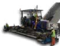
2D, 3D Maskinstyring asfaltering (PCS4000, PCS9000)
