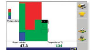
Operator view of temperature mapping
