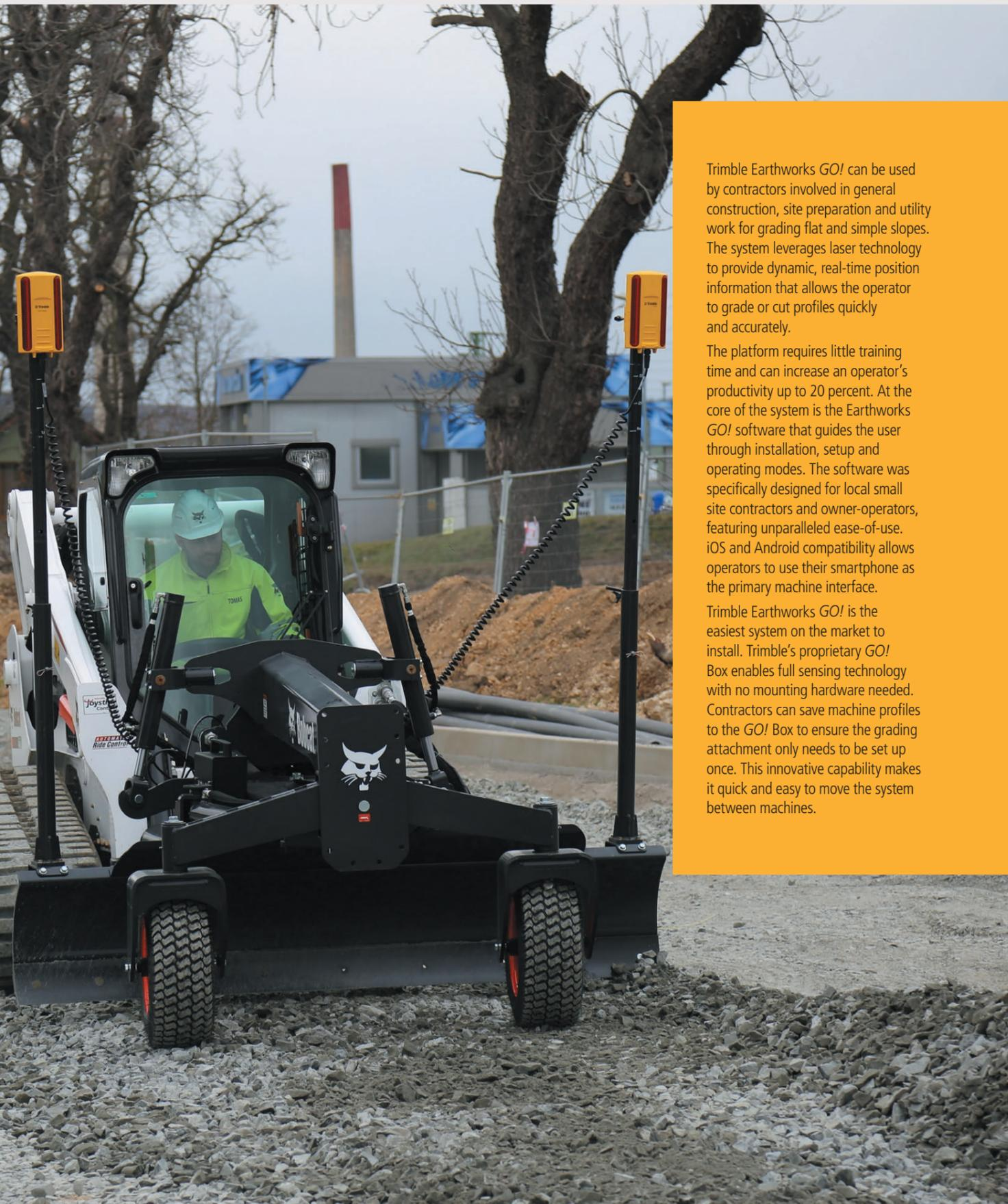
Trimble Earthworks GO! can be used by contractors involved in general construction, site preparation and utility work for grading flat and simple slopes. The system leverages laser technology to provide dynamic, real-time position information that allows the operator to grade or cut profiles quickly and accurately.
