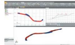
The uncompacted surface designs guide the paver to automatically lay more material above low areas and less material in high areas, anticipating and eliminating longitudinal waves that can occur after asphalt compaction.
