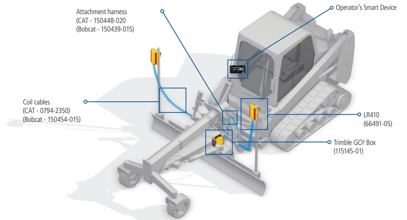
Trimble machine control systems are flexible enough to let you equip your entire fleet—excavators, dozers, scrapers, graders, trimmers, milling machines, compactors, pavers and more—with fully upgradeable technology. Start where you need to start and add as you need to add. Select the best option for the machine and application: sonic, angle sensors, laser, GNSS or total station.
